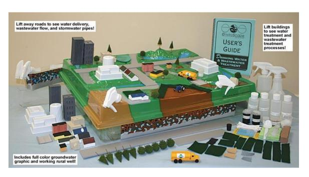
The drinking water and wastewater treatment enviroscape teaches about the water and wastewater treatment processes as well as, septic tanks, groundwater, and storm drains.
